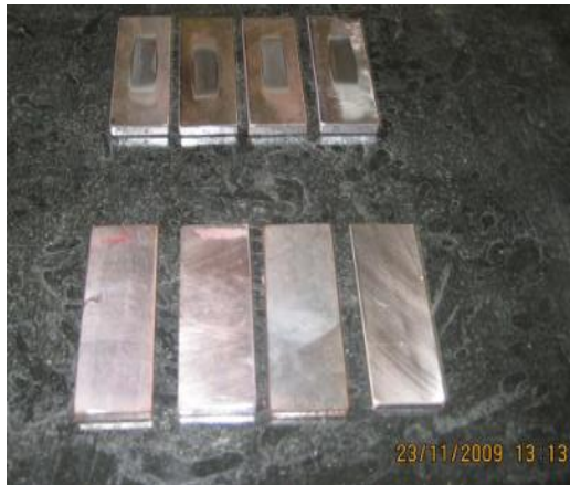
Figure 2. Standard test specimen (75x26x6 mm)
