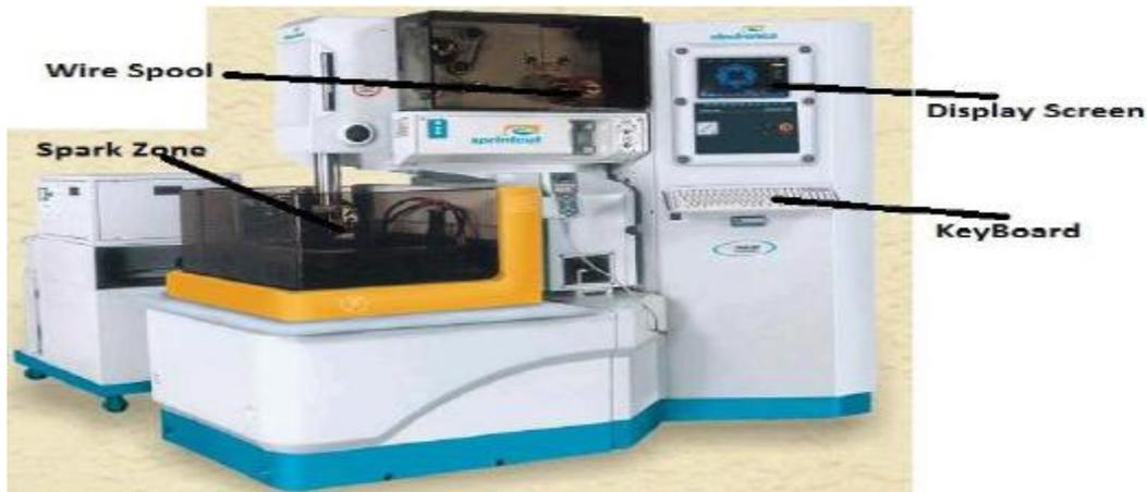
Fig.2: Wire cut EDM (CNC) is used for experimentation
