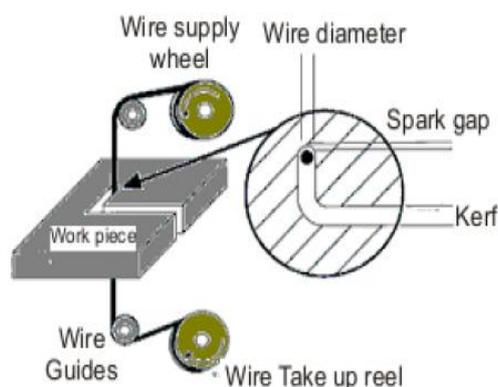
Fig.1: Details of WEDM cutting Gap.
