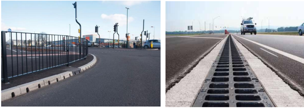
Figure 4 Air port kerb & highway surface drainage system
