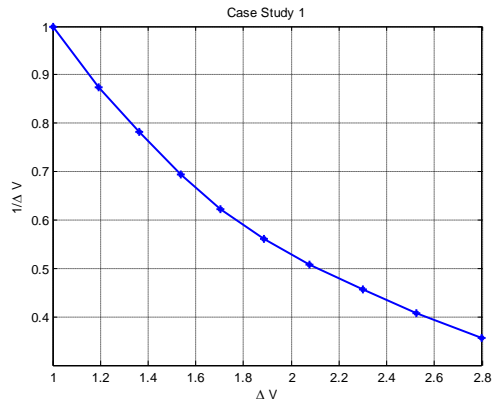
Figure 2: Power Factor versus Voltage Drop.
