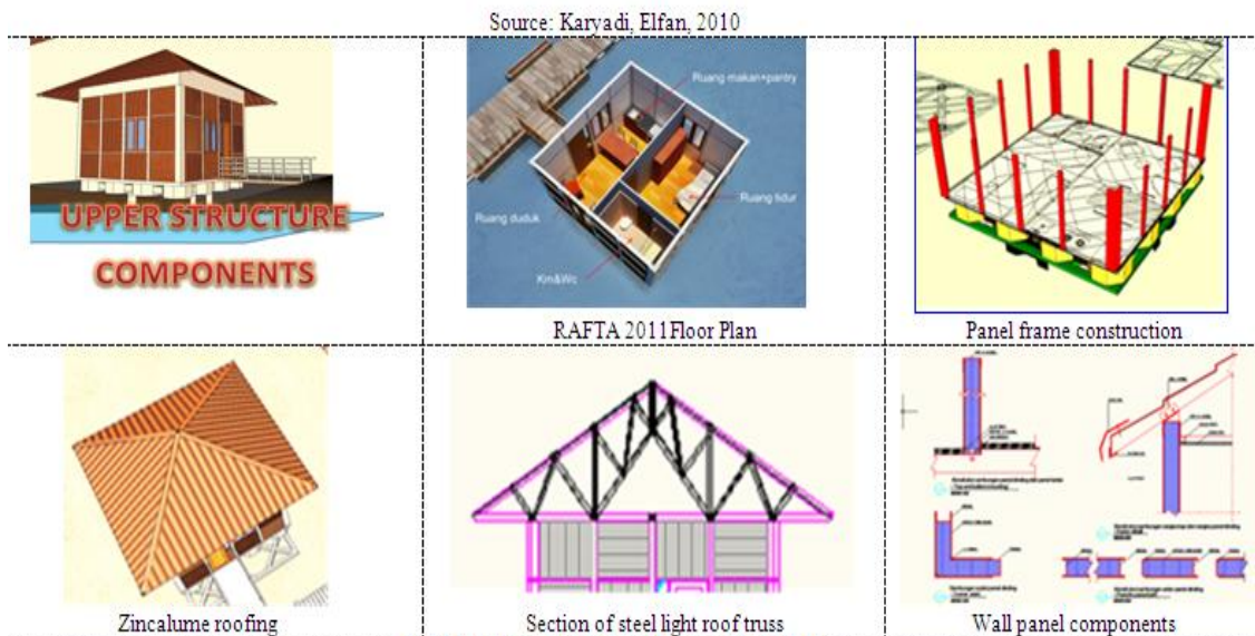
Fig.6. Upper-Structure Construction Component
