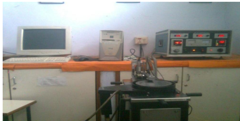
Fig. 4.5 Experimental Setup of Pin-on-disc Tribometer
