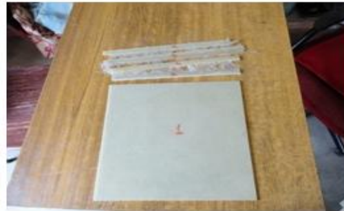
Fig.2- 1wt% nanoclay composite
