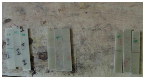
Fig.7- Specimen before flexural test
