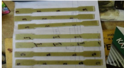
Fig.6- Specimen before tensile test
