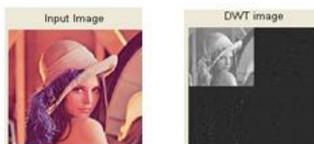
Fig.3. Original host image & decomposed blue channel using wavelet transform
