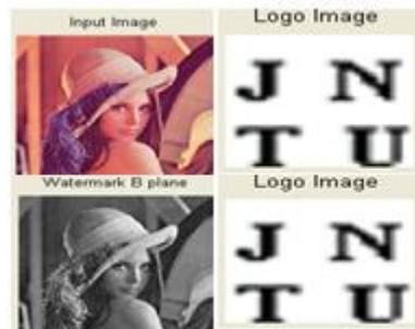
Fig.4. Original host image, original watermark, watermarked image and extracted watermark
