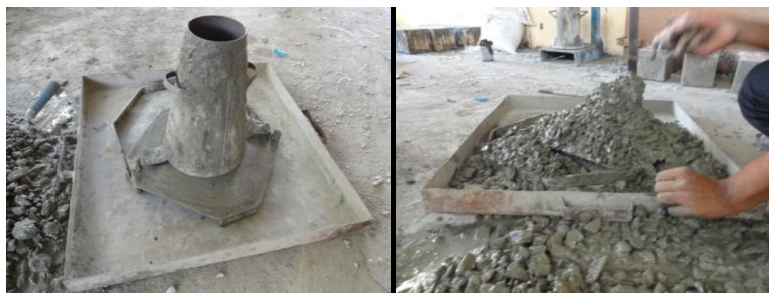
Fig: 2 Slump cone and collapse of concrete after lifting.
