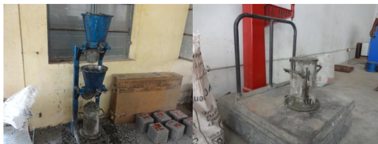
Fig:3 Compaction factor apparatus and weighing of partially weighed concrete
