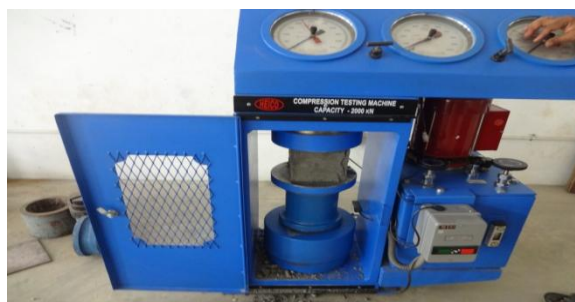
Fig: 5 Testing of cube specimen.
