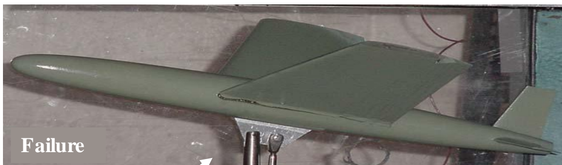
Figure 2. Model airplanes with solid wings during wind tunnel experiments. Angle of attack (A) 0^\circ , (B) 15^\circ ascending and (C) 15^\circ descending.
